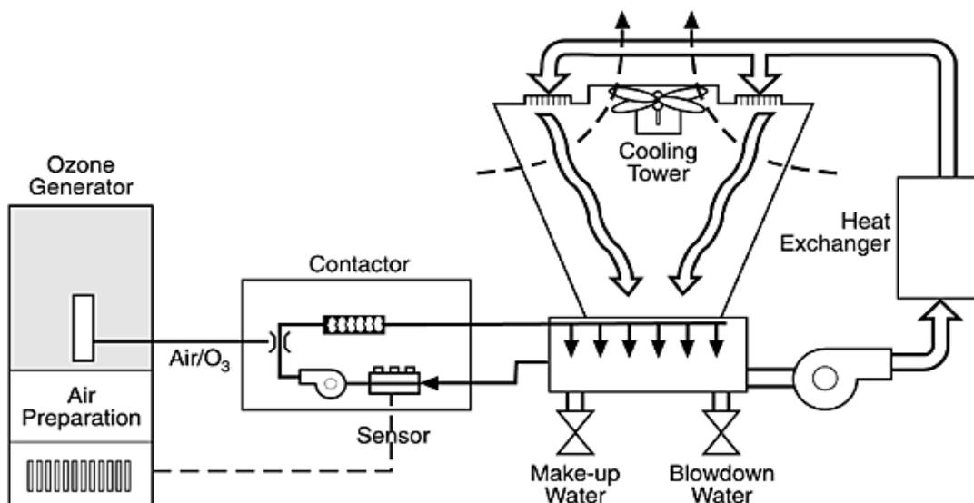
Figure 1 – Ozone Cooling Water Schematic
