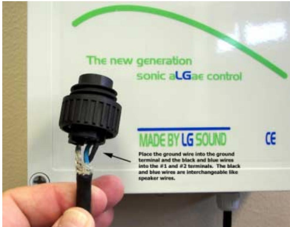
to have plastic in the terminal and also no excess wire outside to short against the ground wire. If these wires cross in the assembly, you are sure to blow one of the two fuses in the device.
