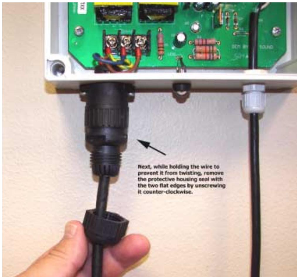
**Step 3:** Now, unscrew the plug from the control box.
