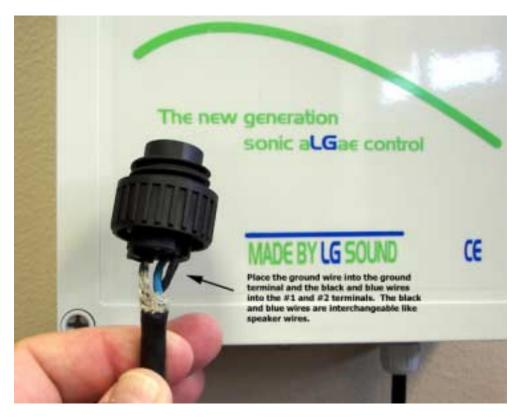
to have plastic in the terminal and also no excess wire outside to short against the ground wire. If these wires cross in the assembly, you are sure to blow one of the two fuses in the device.
