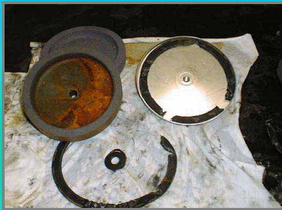
Hypalon diffuser gaskets after 2-yr service in a high-ozone-concentration (8%wt) oxygen-fed ozone application
