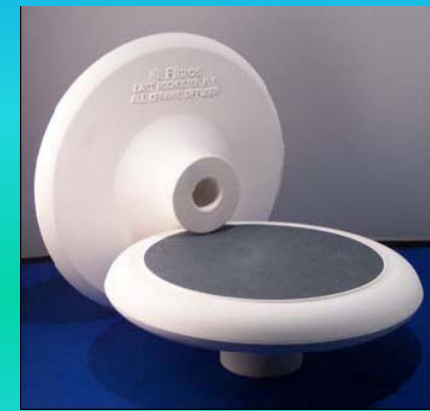
One-piece design is formed of a gas permeable porous alumina diffuser ceramic bonded at high temperature yielding a corrosion resistant product. Stainless steel components, polymer gaskets and cements of any kind have been eliminated.
